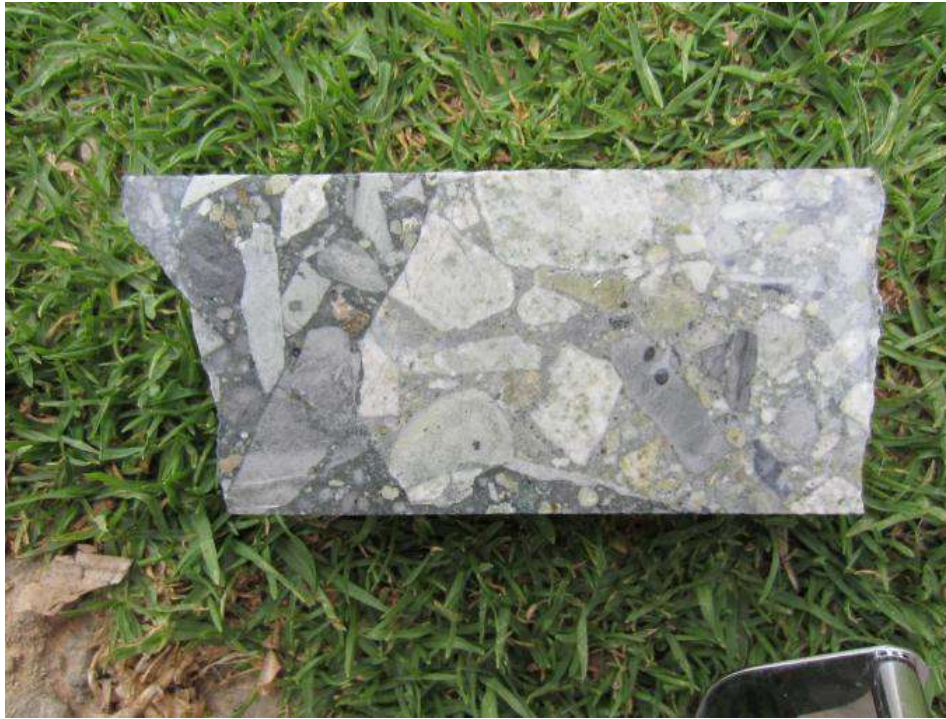
Figure 7.14 Rayo Grande Target, COL-14, 84.0 m, polyphase diatreme/hydrothermal breccia with clasts of massive sulfide. From Turner, 2011.
