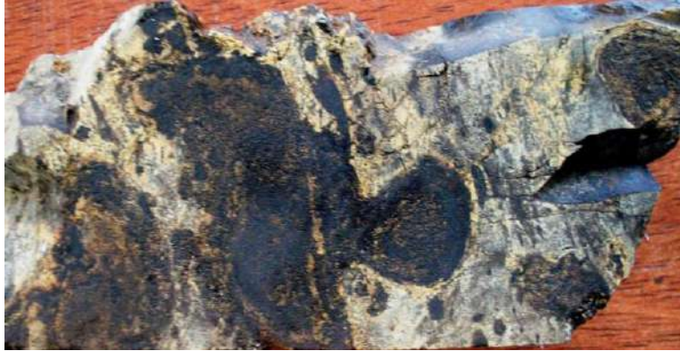
Figure 7.13 Manganese replacement in clastic sedimentary rocks and conglomerate from CPD-04, 21.7m (Turner, 2011)
