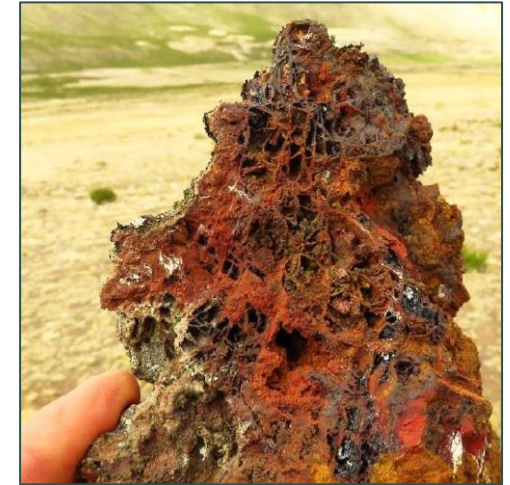
Fine cellular boxworks resulting from intense leaching of primary sulfides.
