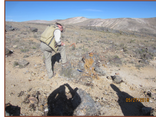
Llamoza Zone: Sample site of subtle vuggy silica structure cutting phreatic breccia returned 18 g/t gold. Structure trends N25W and contains clasts of quartz alunite. View southeast.
